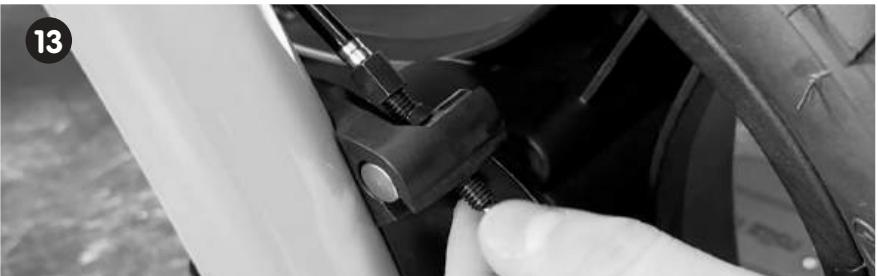
**STEP 13:** Adjust the braking force with the adjustment screw. The brakes should be tight enough that the wheels no longer move when on the parking brake. The parking brake should be easy to release. To increase the braking force, tighten the screw upward. If the tension is too high, the parking brake will no longer engage properly. Adjust carefully to achieve the desired braking performance.
