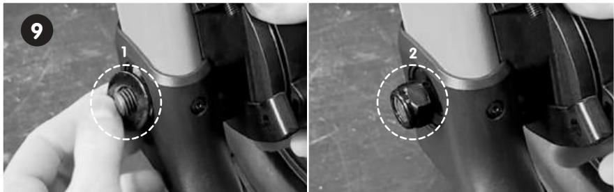
**STEP 9:** Place the ring on the screw (1) and secure it with the nut (2). Do not fasten it yet!
