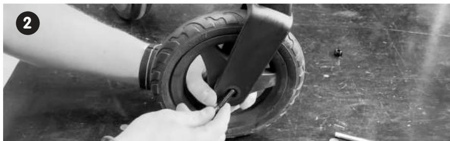
**STEP 2:** Place the new air tire in the fork. Use the axle from the old wheel to secure it in the fork. Repeat step 1 and 2 to replace the other front wheel.
