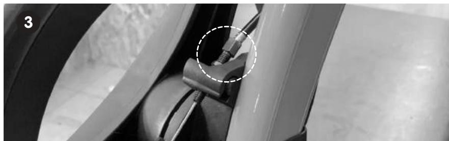
**STEP 3:** To remove the old rear wheels, first loosen up the screw that is holding the brake cable.
