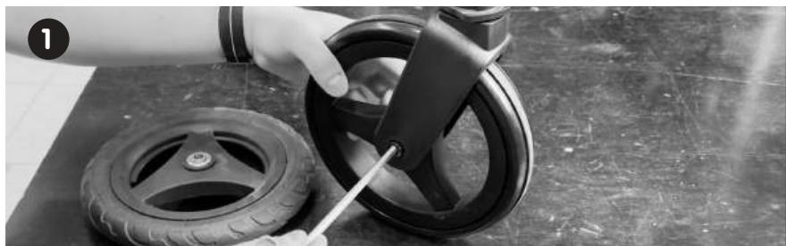
**STEP 1:** To remove the old front wheels, loosen up the axle of the front wheel using allen key size 6. If you have a Rollz rollator made before 2017, you will need allen key size 5. Take the wheel off by pulling it out.
