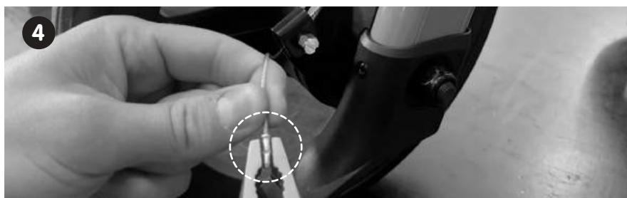
**STEP 4:** Pull the cable cap off sharply using combination pliers. If you don't succeed, try using a bolt cutter or a cable cutter to cut the cap off. However, this may result in split ends making the application of the new cap later more difficult.
