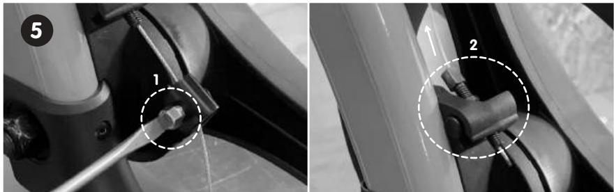
**STEP 5:** Unscrew the cable clamp using the flat head screwdriver and the open-end wrench (1). Remove the cable out of the cable clamp and from the adjustment screw (2).
