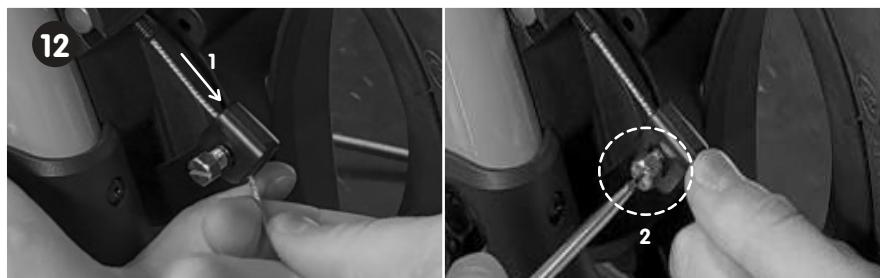
**STEP 12:** Insert the brake cable into the cable clamp (1) and pull it tight with pliers (this will raise the brake lever). Then, use a flathead screwdriver to securely tighten the cable clamp (2).
