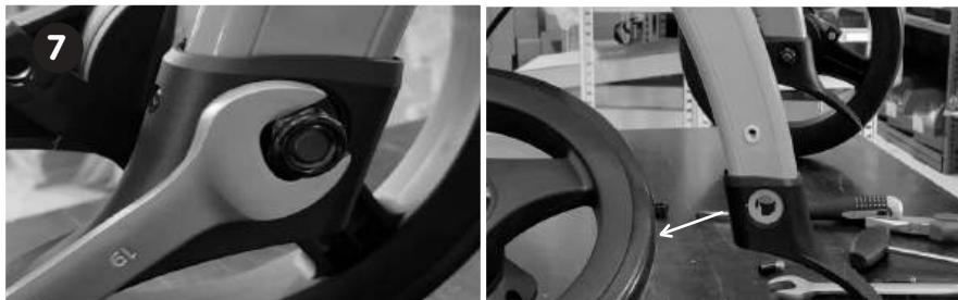
**STEP 7:** Unscrew the nut on the inside of the wheel using ring spanner size 19. Remove the wheel by pulling outwards.
