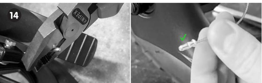
**STEP 14:** Place the new cable cap on the brake cable and squeeze it in place with the combination pliers. Repeat steps 3 to 15 to replace the other rear wheel and perform a safety check.
